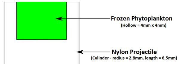
Fig. 1. Schematic showing Projectile structure.
