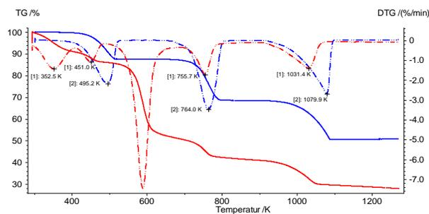
Fig. 2 TG and DTG profiles after hydration at RH=79% in a desiccator: synthetic calciumoxalate monohydrate blue, 2 and *C. gyrosa* red, 1. Solid line TG, dashed line DTG.
