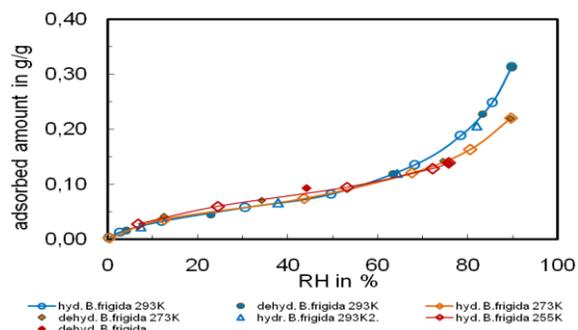
Fig. 4 Hydration/dehydration isotherms of *B. frigida* at 256-293 K.
