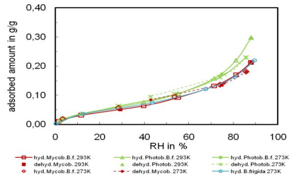
Fig. 5 Hydration isotherms of *B. frigida* at 273 K (blue); hydration/dehydration of the photobiont (green) and mycobiont (red) at 273 and 293 K.
