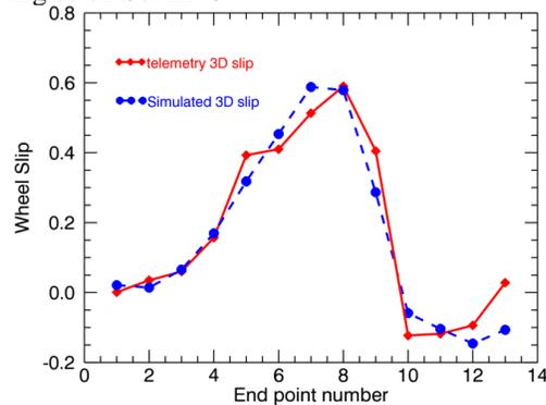
Fig. 3 – Telemetry-based 3D and simulated slips on Sol 2143.
