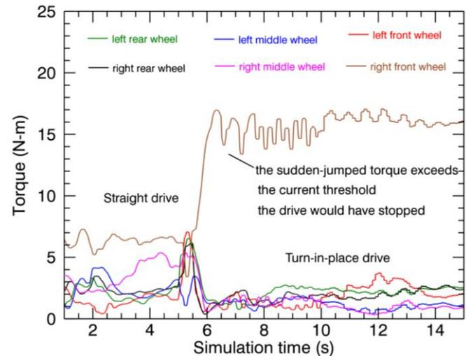
Fig. 6 – Simulated torques for each wheel on Sol 2808 (wheel-drive-actuator current anomaly).
