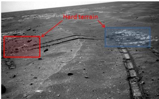
Fig. 1 – Navcam images acquired after the ripple crossing on Sol 2143. Red and blue rectangles represent the hard terrain at the beginning and ending part of the ripple crossing drive, respectively.
