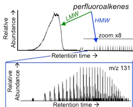
**Figure 1.** Pyr-GCMS results for the diaphragm seal. Total ion chromatogram (top plot) shows both low-molecular-weight (LMW) perfluoroalkenes eluting from the GC column (held at 35 °C in this example) during pyrolysis and significant lower abundances of high-molecular-weight (HMW) perfluoroalkenes that elute from the GC column during ramping to 300 °C. Ion chromatogram for  $m/z$  131 (bottom plot) shows the 6+ homologous series that make up the HMW perfluoroalkene component.
