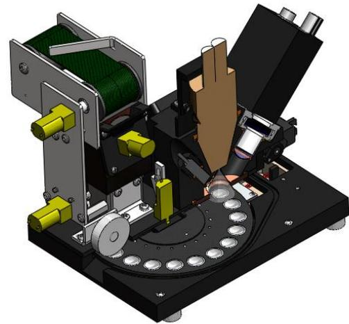
**Figure 2.** Schematic drawing of ODIN. Some components have been removed to allow viewing the inside of the system. Clearly visible are the conveyor belt of the sample transport system, the brush to remove measured aliquots, the turntable with the sample cups, the X-ray source (brown, cut in half), the PMT (right side, facing the sample at an angle) and the heater below the turntable.
