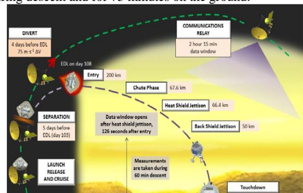
**Fig. 2.** Mission architecture from launch to landing
