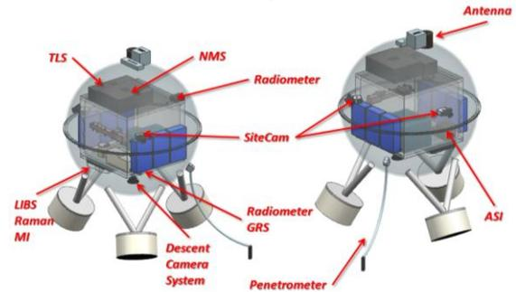
**Fig. 1.** Instrument placement on spacecraft.
