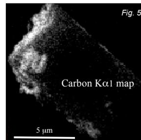
was microtomed, and so, pending further study of the TEM sections, there is a chance that the OM was in the potted butt. A minimum OM mass, estimated from its area in Fig. 5 and assuming  $\sim 0.1$   $\mu\text{m}$  thickness, is  $\sim 5$  pg. If
