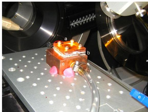
**Figure 1:** The TC stage mounted on the XYZ stage of the  $\mu\text{XRD}$ . The a) sample holder, b) TE module, c) heat sink, d) water hosing, and e) thermocouple are visible in this image.
