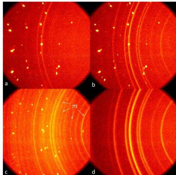
**Figure 2:** GADDS images from the demonstration experiment taken a) immediately, b) after ~2 hours at  $-25^\circ\text{C}$ , c) at  $5^\circ\text{C}$  with secondary mirabilite (m), and d) after equilibration to ambient conditions. The diffraction spots in a and b match the structure of mirabilite, and the Debye rings in a, b, and d match thenardite.
