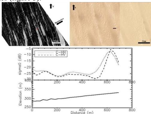
**Fig. 3.** Example profile across a dune in the Great Sand Sea in Egypt. (Top) SIR-C radar backscatter image and corresponding Google Earth® visible imagery are shown. (Bottom) Variation of normalized radar backscatter and elevation with horizontal distance along the dune profile.
