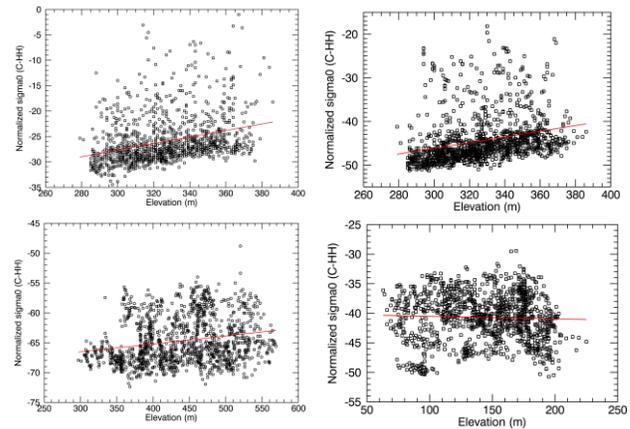
**Fig. 4.** Variation of SIR-C normalized (C-HH) radar backscatter ( $\sigma_0$  in dB) with SRTM elevation (in meters). (Top left) Great Sand Sea (inc=24.8°); (Top right) Great Sand Sea (inc=50°); (Bottom left) Great Sand Sea (inc=65°); (Bottom right) Qattaniya dunes (inc=54°).
