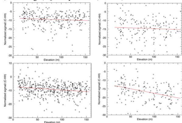
**Fig. 5.** Variation of Cassini SAR normalized (Ku-HH) radar backscatter ( $\sigma_0$  in dB) with assumed elevation (in meters). (Top left) Aztlan; (Top right) Fensal; (Bottom left) Belet; (Bottom right) Shangri-La.
