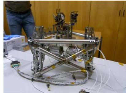
Fig.3. Interface test of seismometry system.
