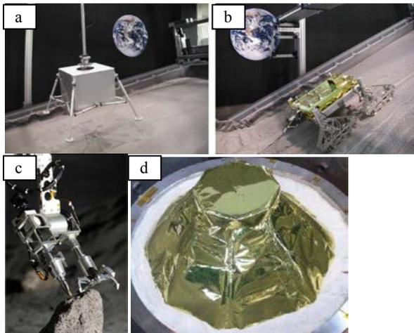
Fig.2. Some examples of technical development of the SELENE-2 system, a) Landing gear, b) Rover system, c) Tool changer on board the rover, and d) BBM of the night survival module.
