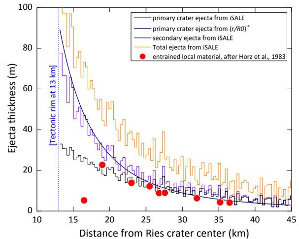
**Fig. 1** Predicted ejecta thicknesses (primary and secondary) in the Ries crater by using iSALE models and comparison with observations from drill cores of the Bunte Breccia [15].
