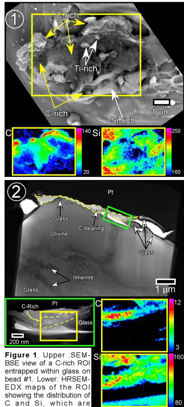
**Figure 1.** Upper :SEM-BSE view of a C-rich ROI entrapped within glass on bead #1. Lower: HRSEM-EDX maps of the ROI showing the distribution of C and Si, which are anticorrelated.
