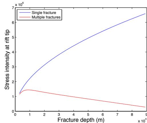
Figure 1. Net stress intensity factor at the crack tip, used to predict fracture propagation, for a single isolated crack in Enceladus' ice shell (blue) and for a fracture in a field of other fractures, e.g., tiger stripes (red).
