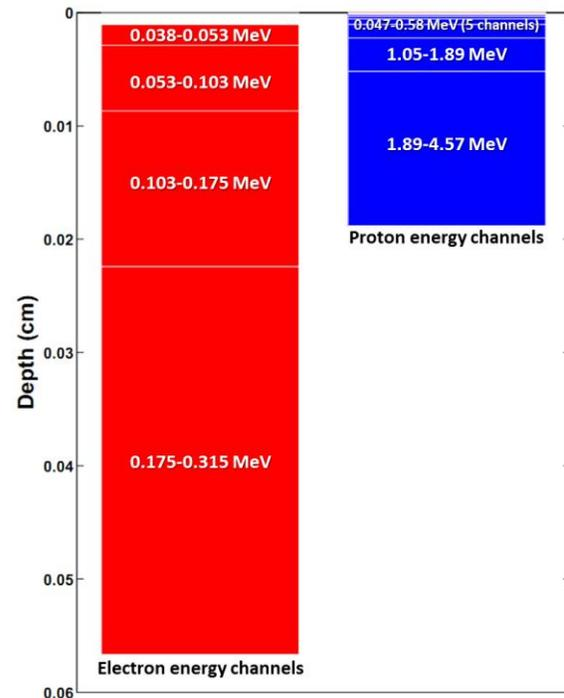
Figure 1: Average regolith penetration depth of electrons (left) and protons (right) in the given energy channels in ACE/EPAM, assuming isotropic incidence.
