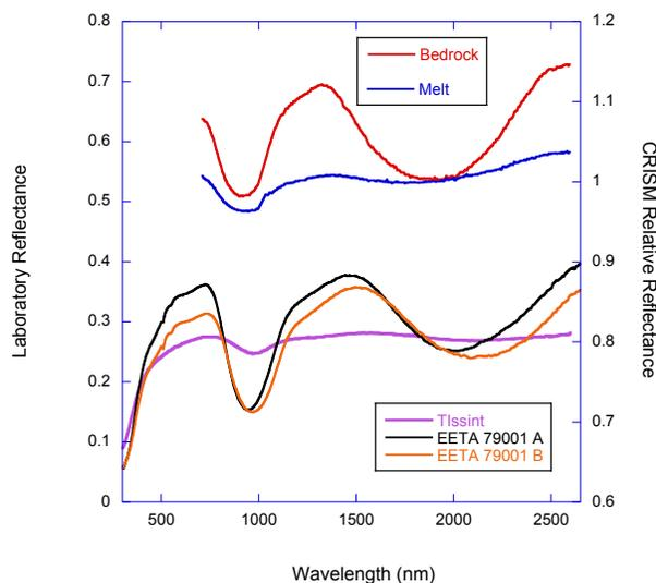
Figure 2. Top spectra are from the central peaks of Alga crater Mars. The bedrock spectrum shows typical
