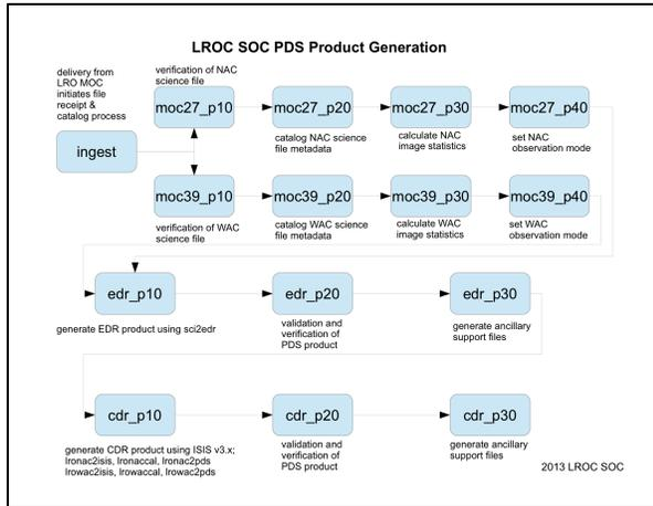
**Figure 2.** This diagram shows the GDS for processing of LROC data.
