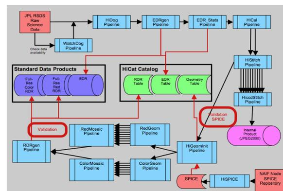
**Figure 1.** This schematic diagram shows the design of the HiRISE GDS used to process raw PDS EDR images into calibrated, map-projected data products.
