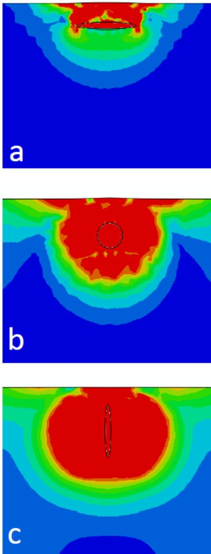
Figure 1. The von mises stress for a) a sill like intrusion b) circular intrusion and c) dike like intrusion. The red shows von mises stresses greater than the yield stress of 1MPa.
