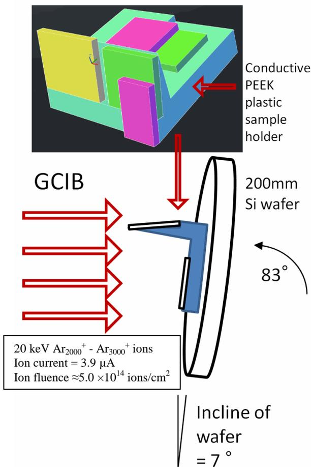
Figure 1. GCIB irradiation geometry
