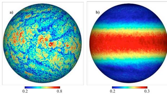
**Figure 3:** **a)** Instantaneous and **b)** time-averaged temperature at radial level  $r=0.992r_o$ , where  $r_o$  is the outer ocean boundary. Dimensionless temperatures measured relative to the temperature contrast between the inner and outer ocean boundaries.
