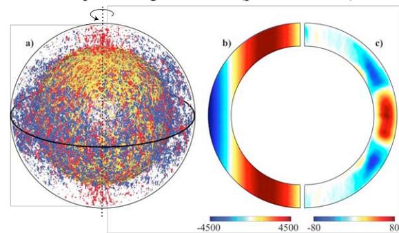
**Figure 2:** a) Instantaneous isosurfaces of axial vorticity. Time-averaged, axisymmetric b) zonal flows and c) radial velocity field. Dimensionless velocities measured in Reynolds number units,  $Re=UD/v$ .
