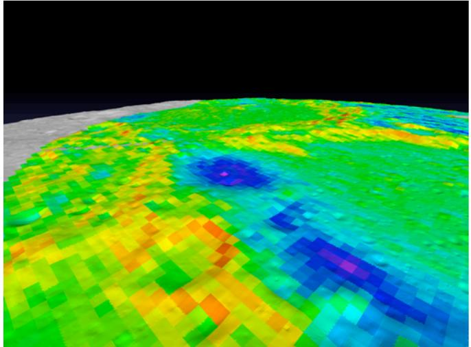
Diviner Channel 9 brightness temperatures for a portion of Hermite crater in the lunar north polar region obtained near midnight near winter solstice. The spatial resolution is 2 km. The purple regions have brightness temperatures approaching 20K.
