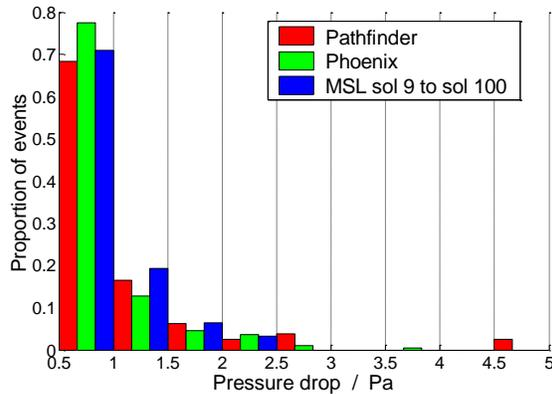
**Fig 1.** Magnitude distribution of pressure drops with magnitude > 0.5 Pa. Pathfinder data taken from [7] and Phoenix data from [4].
