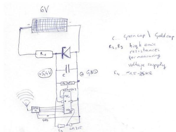
Illustration: circuit diagram of the Micro Mars Probe
