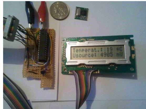
**Illustration: Working prototype of the probe (Size compared to a quarter dollar). Instead of the LCD-display there would be a radio transmission system attached to the probe. On the top right, next to the coin is the Radio Frequency module (for wireless data transmission between the probes) which will be attached. Measured values: Temperatures in degrees Celsius and voltage supply.**
