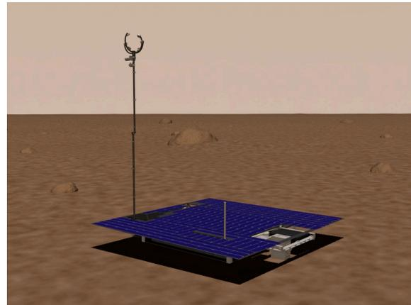
**Figure 1 MSCL with the mast fully deployed after dropoff from parent rover.**
