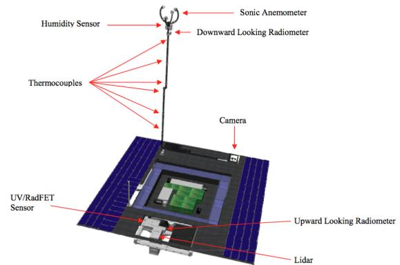
**Figure 2** The MSCL instrumentation layout.
