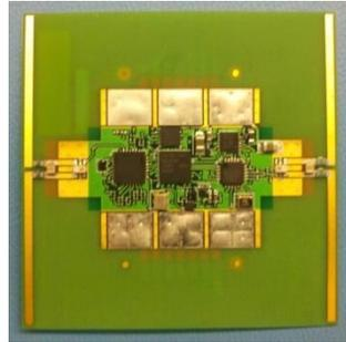
Figure 1. Current ChipSat Bus
