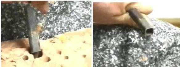
Figure 1: Square cross-section bit of a percussive drill.
