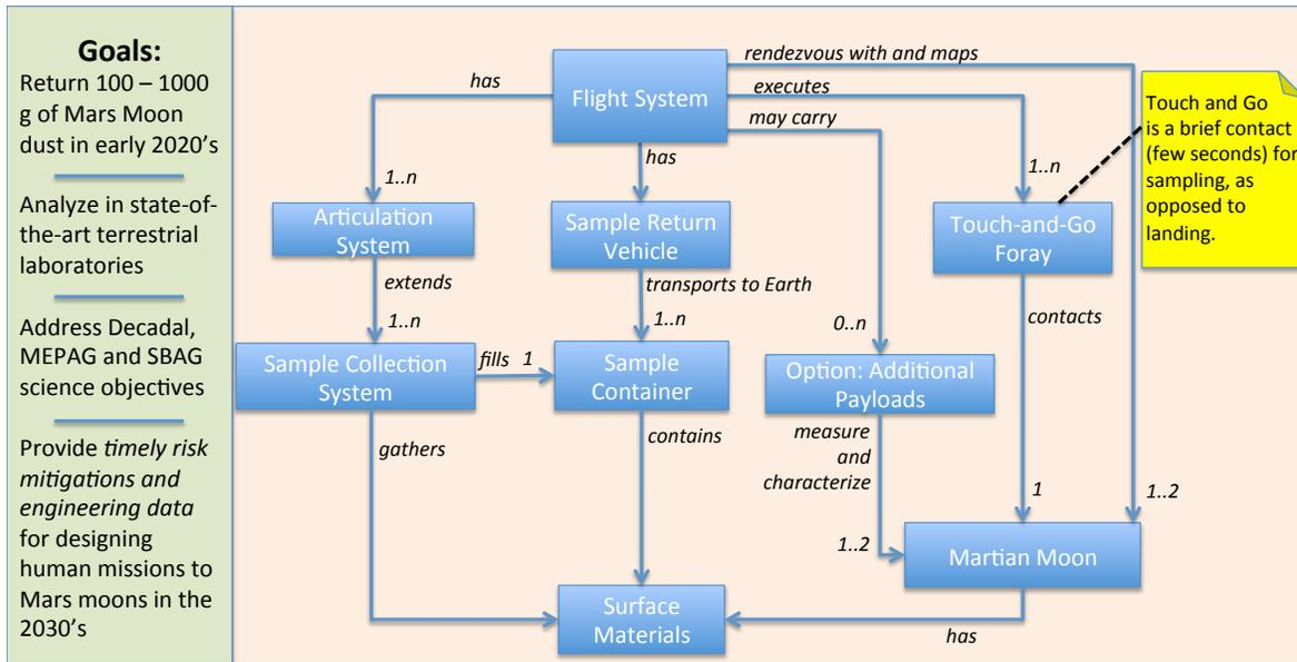
**Figure 1: Block Diagram of Key Elements for a Mars Moon Sample Return Mission**
