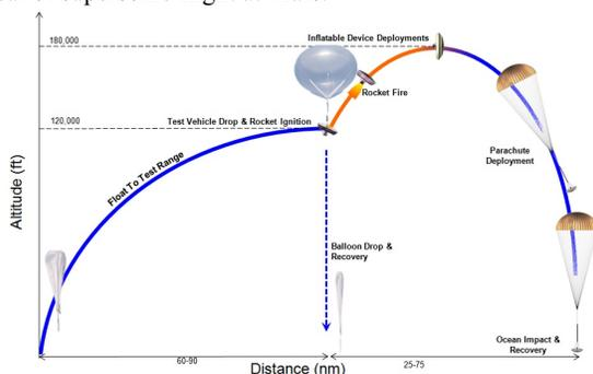
**Figure 1. Basic concept of the Supersonic Flight Dynamics Test architecture.**
