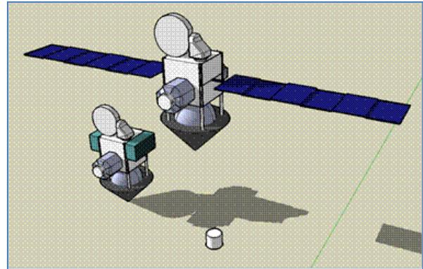
Figure 2: Sample containment Capsule (bottom), folded return vehicle (middle), deployed return vehicle (top).
