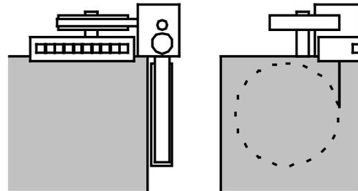
Figure 1: Top view (left) and side view (right) of sample collection tape mechanism with 10-cell bag mechanism.
