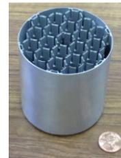
Figure 3: Example sample cache canister.
