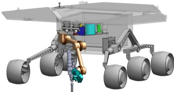
Figure 1: Sample Acquisition and Caching on a MER-class rover.
