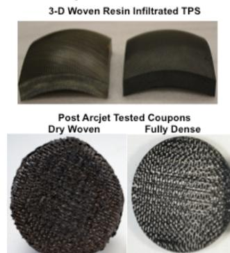
Figure 2. Woven TPS comparable to Fully Dense Carbon Phenolic as well as mid-density TPS has been manufactured and tested both mechanically and thermally.
