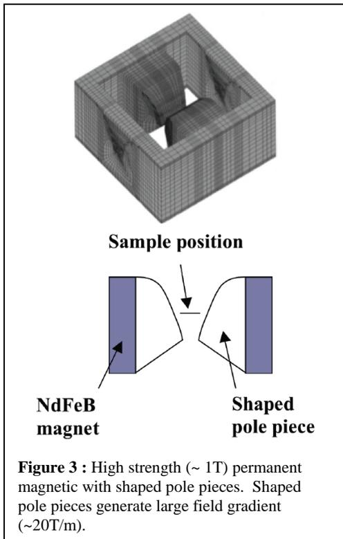
**Figure 3 :** High strength ( $\sim 1\text{T}$ ) permanent magnetic with shaped pole pieces. Shaped pole pieces generate large field gradient ( $\sim 20\text{T/m}$ ).
