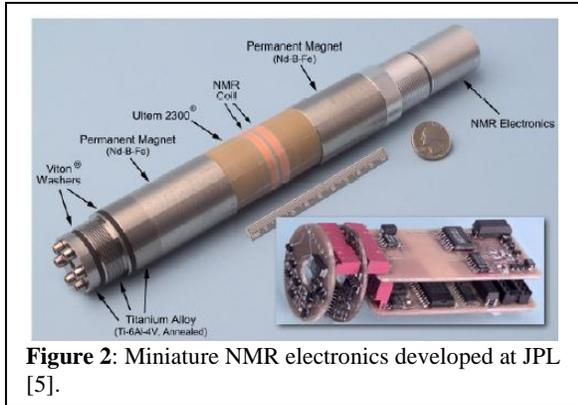
**Figure 2:** Miniature NMR electronics developed at JPL [5].
