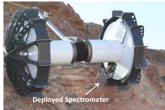
**Figure 1:** Axel deploying and acquiring infrared spectroscopic measurements and microscopic images from its instrument bay on exposed strata ( $40^\circ$  slope).
