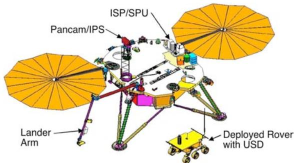
Figure 1. Lander concept with small fetch rover.
