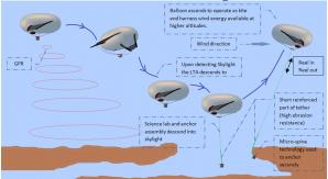
Figure 3: Searching, anchoring and harvesting energy from airborne wind energy.
