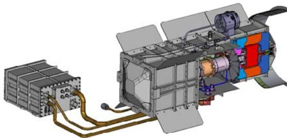
operate for years in extreme cold environments, the use of ASRGs is enabling. After being coupled to the power bus via enable plugs, the full ASRG power output is fed into the lander power bus at all times. ASRG internal power shunting capability is necessary for preflight integration activities, but once it is switched in to the lander power bus, all excess ASRG power is managed via lander shunts. This shunting is
