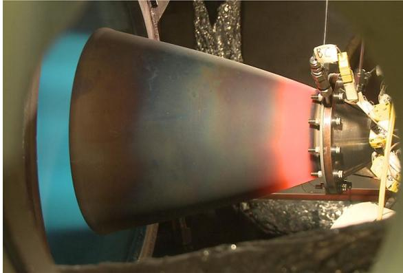
**Figure 3. Regeneratively-Cooled TR408 LOX/LCH4 Engine**
