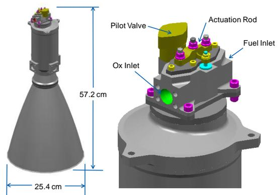
**Figure 2. MAPS Main Engine (5.3 kN)**
