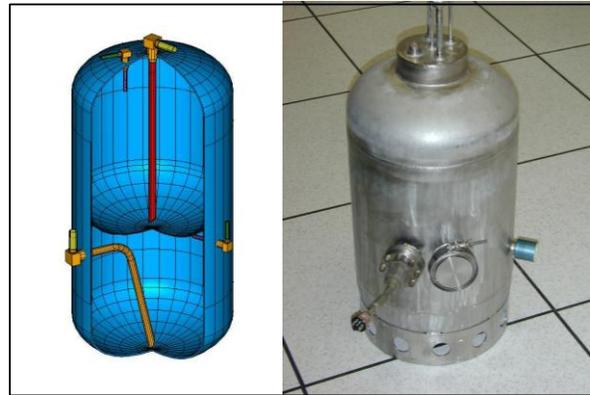
**Figure 3 – Common bulkhead tank envisioned for ascent vehicle keeps propellants at same temperature until launch.**
