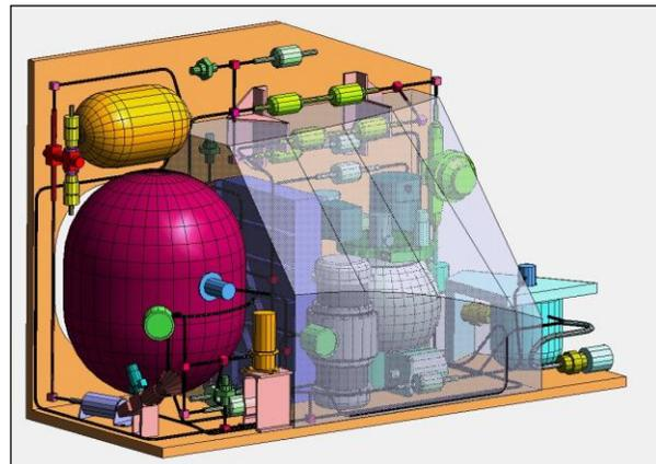
**Figure 2 - Early propellant production concept called the Propulsion Utilization of Martian Produced Propellants (PUMPP) shows highly integrated system.**
