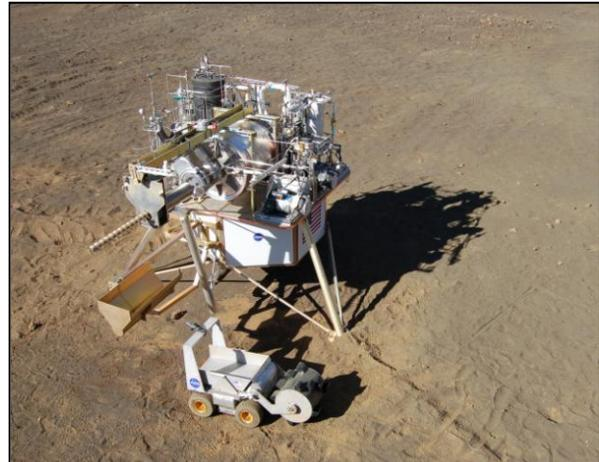
**Figure 1 – Precursor In-Situ Lunar Oxygen Testbed represents a self-contained approach developed for lunar resources.**
