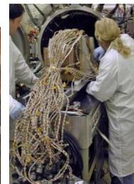
Figures 2 and 3 MER WEB and the MER jungle of wires connecting the WEB to loads located at the extremities of the rover.
