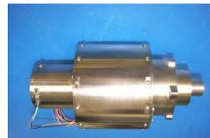
Figure 4 Low Temperature MSL Class Motor, Gearbox combination capable of operating at temperatures as low as -240C developed by NASA ETDP.
