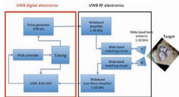
Fig. 1: UWB radar block diagram
