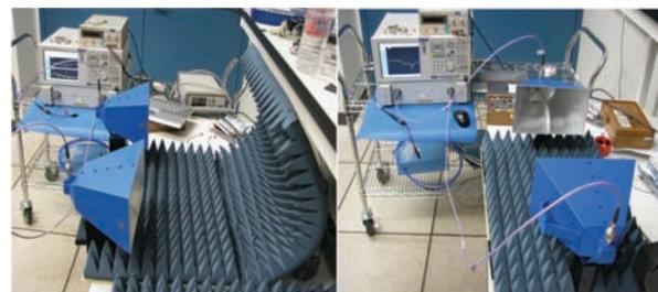
Fig. 2: UWB antenna cross talk and gain calibration at 1-10 GHz
