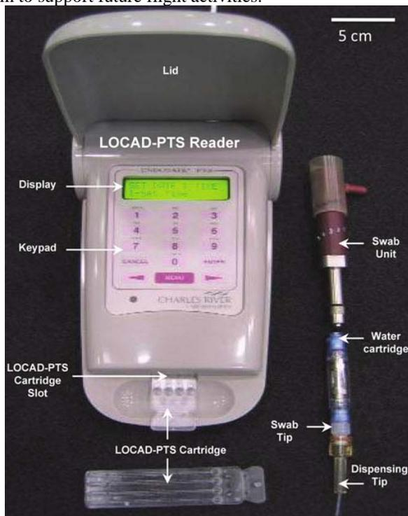
**Figure 1. Flight instrument and disposables for LOCAD-PTS [1].**
