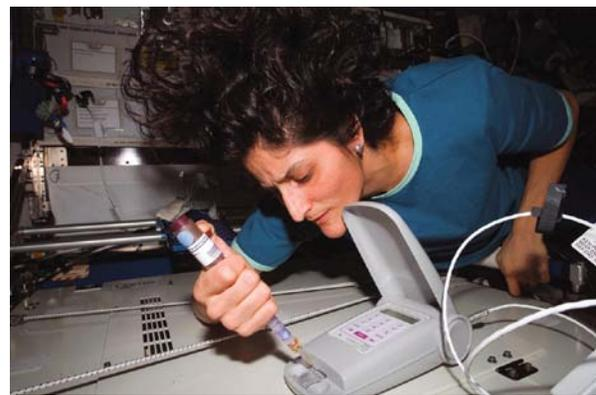
**Figure 2. Sample being loaded into LOCAD-PTS [1].**
