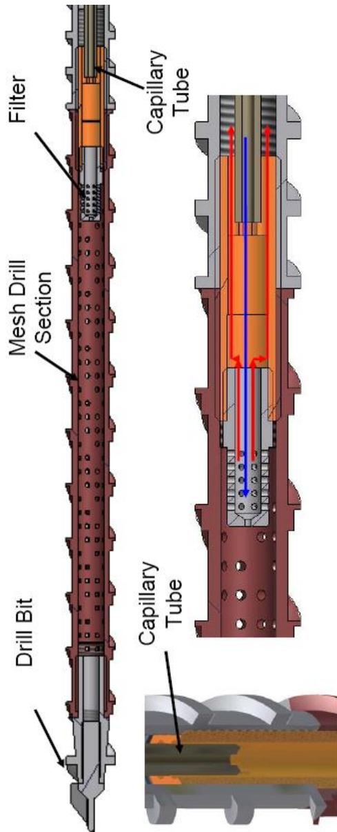
**Figure 2.** Details of the ‘Sniffing’ part of the drill string.
