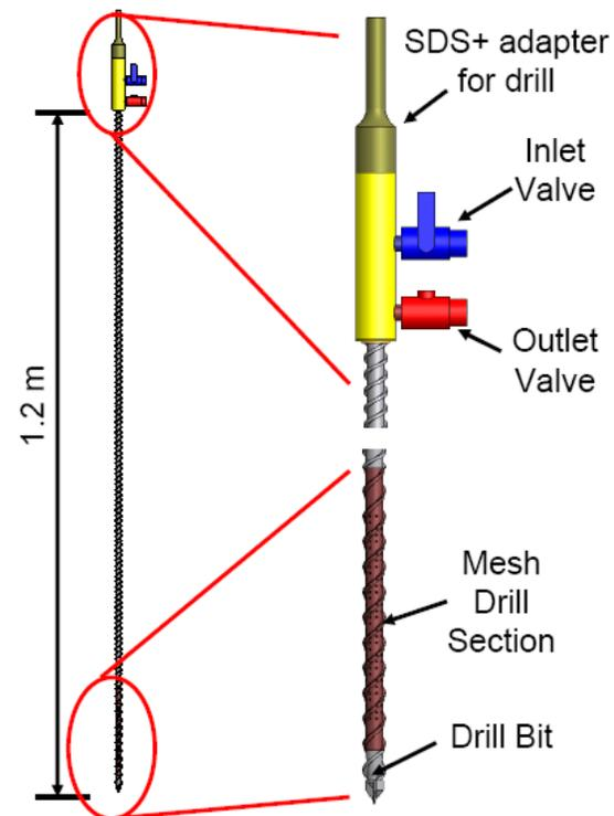
**Figure 1. View of the Sniffer drill.**
