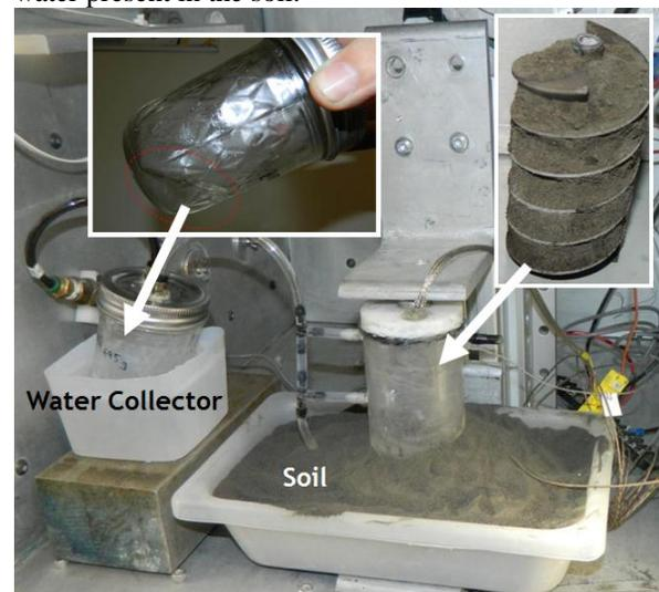
Figure 4. MISWE water extraction system being tested in Mars chamber.
