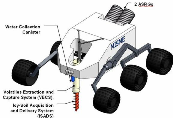
**Figure1. Mars In-Situ Water Extractor (MISWE).**
