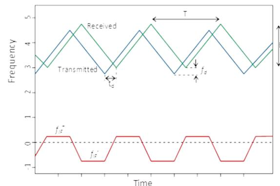
**Fig 1.** Linearly frequency modulated transmitted beam and returned signal, and the resulting intermediate frequency (IF) of the homodyne signal.
