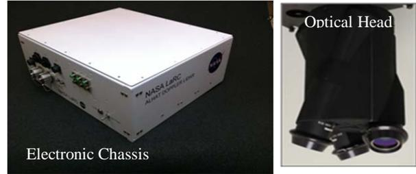
**Fig. 3.** Prototype Doppler lidar system consisting of an electronic chassis and an optical head. All the lidar components, including transmitter laser, receiver, and real-time processor, are housed in the electronic chassis. The optical head, consisting of three transmit and receive lenses, is rigidly mounted to the platform body with a clear view of the ground and connected to the electronic chassis through a long fiber optic cable.
