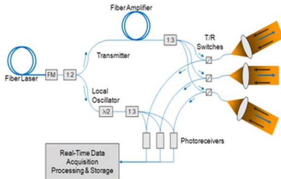
**Fig. 2.** Doppler lidar system configuration illustrating three transmitted beams and their corresponding receivers providing line-of-sight velocity and range measurements in three different directions.
