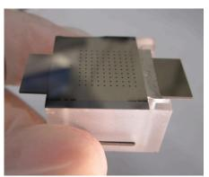
**Figure 1:** Prototype MEP thruster, feed system, and propellant - only 19x19x14 mm.
