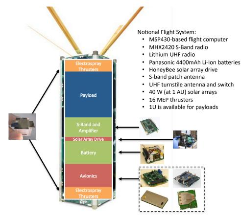
Figure 2: CubeSat and MEP technology could enable a 3-4 kg spacecraft capable of flight between Earth and Mars.
