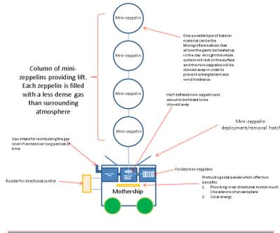
Figure 1: A simple architectural diagram of the system (zoom for details). The mothership here is the rover which can deploy smaller bots
