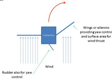
Figure 2: Aileron/solar panels and rudder flight control. The mothership here is the robotic rover that can deploy smaller bots to explore the environment
