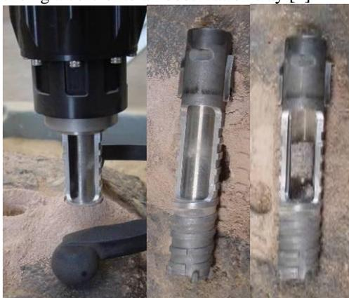
**Figure 4. The Preview Bit. Left: after reaching the target depth, break-off tube is rotated to shear and capture the core. Once the tube is fully closed (Center), the core cannot fall out. To view the core, the inner break-off tube is rotated back to expose it. (Right)**
