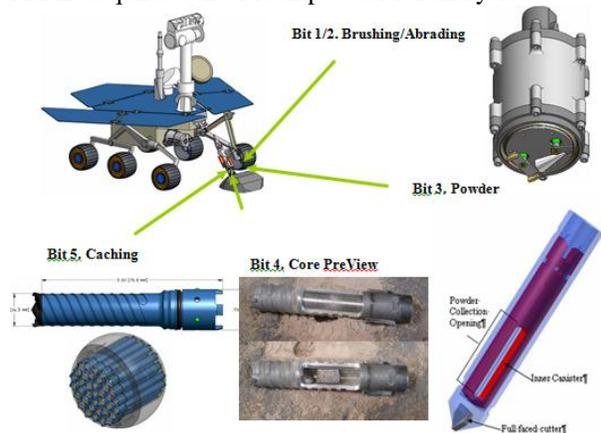
**Figure 1. 5in1 approach: 5 unique bits for different tasks deployed from the same drill.**
