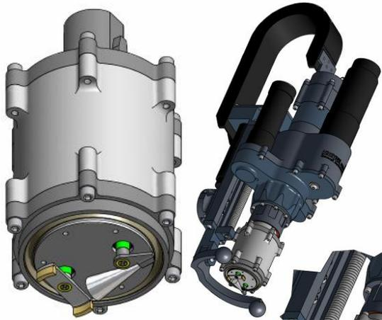
**Figure 3. Concept of Brushing/Abrading Tool (BAT) based on MER Rock Abrasion Tool.**
