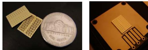
Figure 2: The two symmetrical  $\mu$ -CIT array half-structures before bonding (left); the complete  $\mu$ -CIT array obtained after bonding the two half-structures and mounting them on an Au-coated PCB substrate (right).
