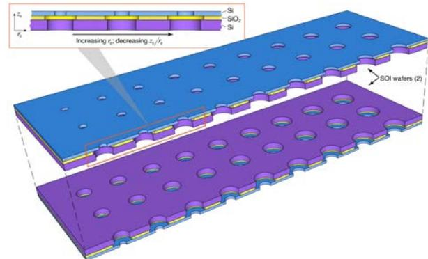
Figure 1: A cross-sectional schematic of a  $\mu$ -CIT array fabricated in an SOI substrate.
