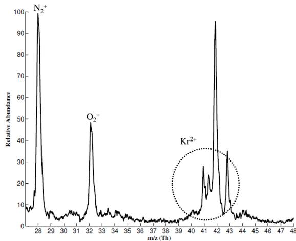
Figure 3: Experimental mass spectral data from a single trap ( $z_0/r_0 = 0.97$ ) in the  $\mu$ -CIT array. Axial modulation was used to obtain better-than-unit mass resolution. Krypton doubly charged ions correspond to masses 82, 83, 84 and 86.
