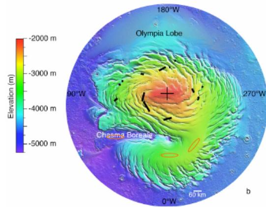
*Figure 1: Approximate MER landing ellipse (red ovals) (100km x 20km) placed in several locations on the Boreale Lingula or in Chasma Boreale show that precision guided entry is not required. Elevations are well below the -1.3km bound for the EDL system.*
