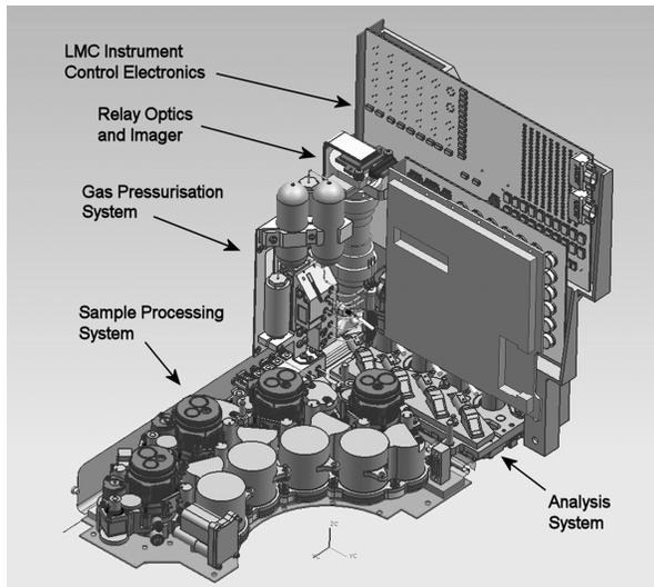
**Figure 2:** CAD image of LMC instrument design, correct as of December 2011 showing the various component subsystems of the instrument. The design mass is 4.7kg including contingency (for a four module / sample system).
