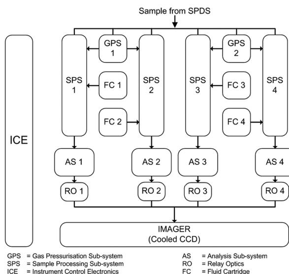
**Figure 1:** Scheme illustrating basic systems architecture of the LMC instrument.
